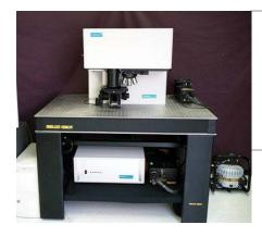
The Microscope / MACROscope® is a unique scanning laser confocal imaging system that uses our proprietary widefield MACROscope® laser scanning technology that allows high-resolution imaging of large specimens and a high level of customization. The addition of a microscope scan head gives very high-resolution laser confocal imaging. No need to purchase two separate systems to fully scan large and small samples.
